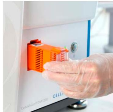
**1** The microscope is replaced by a digital imaging system that automatically locates and then captures digital images of cells from barcoded slides.
